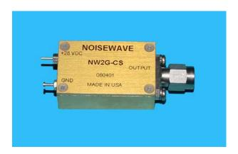
NoiseWave announces the immediate availability of the new NoiseWave NW2G-CS coaxial noise source. Available in 15 and 30 dB ENRs (Excess Noise Ratios), the NW2G-CS is ideal for noise figure measurements and built in test applications. The unit features a small profile housing of 0.75 by 0.5 by 1.25 in excluding connectors, ideal when space is at a premium.
