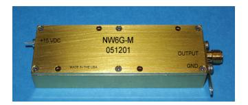
NoiseWave announces the immediate availability of the NW-6GM amplified noise model. The unit features broadband frequency coverage from 10 MHz to 6 GHz ideal for wireless test applications, covering all major wireless applications. Power out is 0 dBm and the unit features a flatness of +/- 2.0 dB. The unit is internally regulated and operates with +15 Vdc and draws 200 mA.
